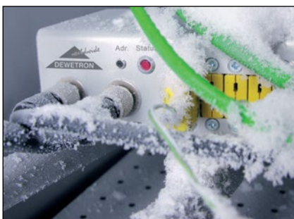
Extensive temperature tests (-40 to +70 °C)
